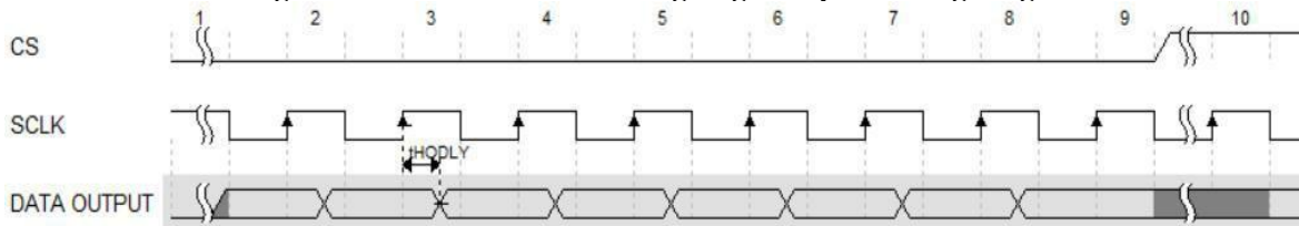
Figure 12-3. HSOD=1 Data Rising Edge Output Timing Diagram
